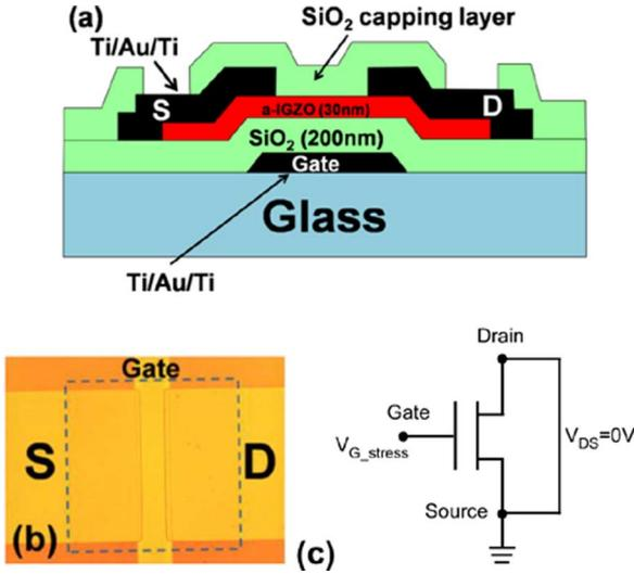
Fig. 1. (a) Cross-sectional and (b) top view of the RF sputter a-IGZO TFT device used in this study. Dash square indicates the region of a-IGZO active layer. (c) The schematic of the circuit setup used for steady state BTS experiments.
