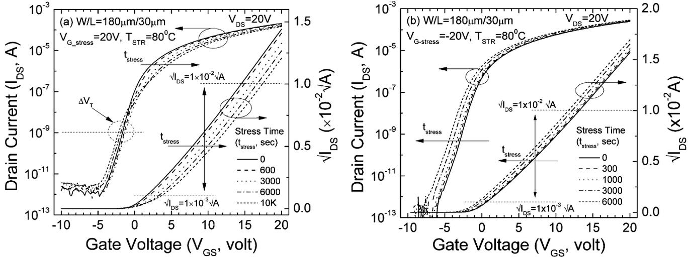
Fig. 8. The evolution of RF sputter a-IGZO TFT transfer characteristics for (a) positive BTS ( $V_{G\_stress} = 20$  V) and (b) negative BTS ( $V_{G\_stress} = -20$  V). For both experiments, the stress temperature,  $T_{STR}$ , is  $80^\circ\text{C}$ .
