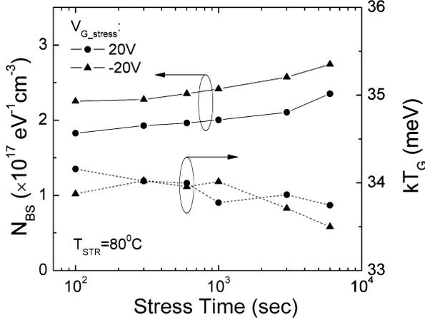
Fig. 10. Density of bulk-states ( $N_{BS}$ ) and characteristic temperature of conduction-band-tail-states ( $T_G$ ) as a function of stress time ( $t_{stress}$ ) for both positive ( $V_{G\_stress} = 20$  V) and negative ( $-20$  V) BTS.
