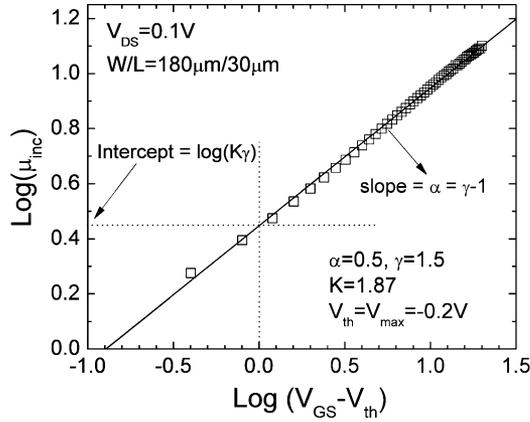
Fig. 6. The log-log plot of the incremental field-effect mobility ( $\mu_{inc}$ ) as a function of the effective gate voltage ( $V_{GS} - V_{th}$ ). The  $V_{th}$  is extracted from  $V_{max}$  in Fig. 4. Solid line is the linear fit to the experimental data (symbol:  $\square$ ).
