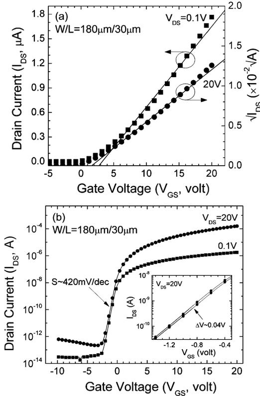
Fig. 3. Transfer curves of a-IGZO TFT in (a) linear and (b) semi-log scales. (Inset, b) The TFT hysteresis measured at  $V_{DS} = 20$  V;  $\Delta V$  is the shift in sub-threshold properties. Symbol (●) and (■) represent the saturation ( $V_{DS} = 20$  V) and linear ( $V_{DS} = 0.1$  V) region properties, respectively.
