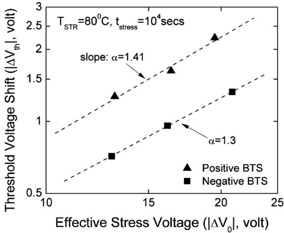
Fig. 12.  $\Delta V_{th}$  as a function of effective stress voltage ( $\Delta V_0$ ) for positive (symbol:  $\blacktriangle$ ) and negative ( $\blacksquare$ ) BTS. Dash lines are the linear fit to the experimental data.
