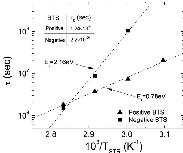
Fig. 15. Characteristic trapping time  $\tau$  for positive (symbol: ▲) and negative (■) BTS as a function of  $1/T_{STR}$ . ( $T_{STR}$  range: 50 °C–80 °C). Dash line: numerical fit to (18).
