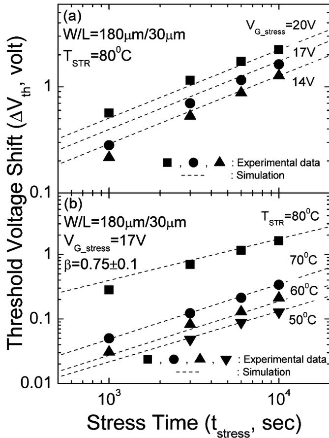
Fig. 13.  $\Delta V_{th}$  vs stress time ( $t_{stress}$ ) for various (a) positive stress voltages ( $V_{G\_stress} = 20$  V, 17 V and 14 V,  $T_{STR} = 80$  °C) and (b) temperature ( $T_{STR} = 50$  °C  $\sim$  80 °C,  $V_{G\_stress} = 17$  V). Symbols represent the experimental data while dashed lines are the simulation fits to stretched-exponential model ((16)).
