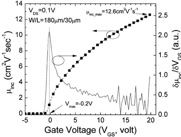
Fig. 4. Symbol (■): The incremental field-effect mobility ( $\mu_{inc}$ ) of a-IGZO TFT extracted by using (5). The differentiation of  $\mu_{inc}$  ( $\delta\mu_{inc}/\delta V_{GS}$ , solid line) is also shown.  $V_{max}$  represents the  $V_{GS}$  with maximum  $\delta\mu_{inc}/\delta V_{GS}$ .
