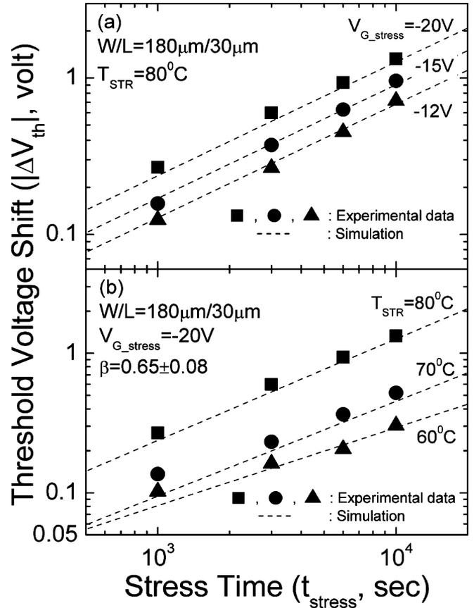
Fig. 14.  $\Delta V_{th}$  vs stress time ( $t_{stress}$ ) for various (a) negative stress voltages ( $V_{G\_stress} = -20$  V,  $-15$  V and  $-12$  V,  $T_{STR} = 80$  °C) and (b) temperature ( $T_{STR} = 60$  °C  $\sim$  80 °C,  $V_{G\_stress} = -20$  V). Symbols represent the experimental data while dashed lines are the simulation fits to stretched-exponential model ((16)).
