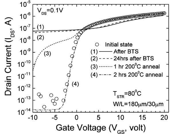
Fig. 11. Recovery of the a-IGZO TFT electrical instability after thermal annealing. (1) TFT transfer properties after severe BTS condition ( $V_{G\_stress} = 27$  V,  $T_{STR} = 80$  °C, 40 Ks); (2) 24 hr of storage under room temperature after BTS; (3) after 1 hour and (4) 2 hours of thermal annealing (200 °C) in air.
