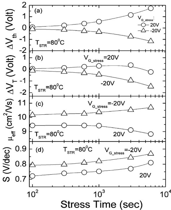
Fig. 9. (a)  $\Delta V_{th}$ , (b)  $\Delta V_T$ , (c)  $\mu_{eff}$  and (d)  $S$  as a function of stress time ( $t_{stress}$ ) for both positive ( $V_{G\_stress} = 20$  V) and negative ( $-20$  V) BTS. Symbols represent the experimental data and lines are for aid of eye.
