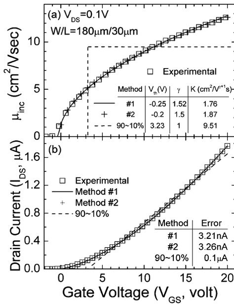
Fig. 7. The calculation of (a)  $\mu_{inc}$  and (b)  $I_{DS}$  based on different models/extraction methods used in this study. Method #1 (solid line) is conducted in Fig. 5. Method #2 (+) is illustrated in Fig. 6. The 90%~10% method (dash line) is conducted based on the standard MOSFET equation ((1)). Symbol ( $\square$ ): experimental data.
