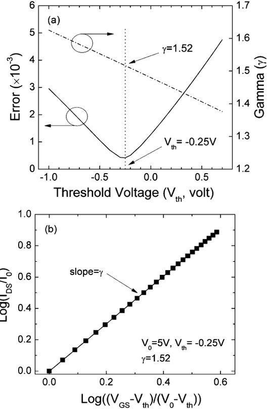
Fig. 5. (a) Variation in  $\gamma$  of the experimental I-V data in above threshold region as a function of  $V_{th}$ . A reference gate voltage  $V_0$  of 5 V is used for parameter extraction. Also shown is the rms error of the least-square fit to the log of drain current ratio ( $\text{Log}(I_{DS}/I_0)$ ). (b) Example of the actual linear fitting plot to (13) at  $V_{th}$  with minimum error ( $-0.25 \text{ V}$ ).
