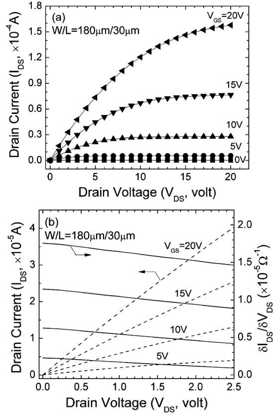
Fig. 2. (a) Output characteristics of RF sputter a-IGZO TFT. (b) A zoom-in plot of the output characteristics (dash curves) near origin ( $V_{DS} = 0 \sim 2.5$  V); the derivative of  $I_{DS}$  vs.  $V_{DS}$  ( $\delta I_{DS}/\delta V_{DS}$ , solid curves) are also shown.
